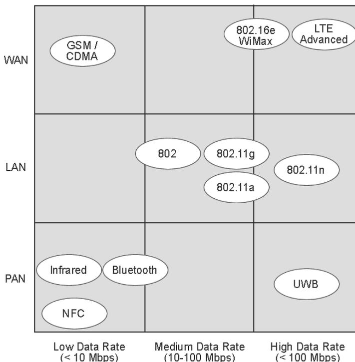
Figure 1: An overview of wireless communication technologies (image courtesy [1])
